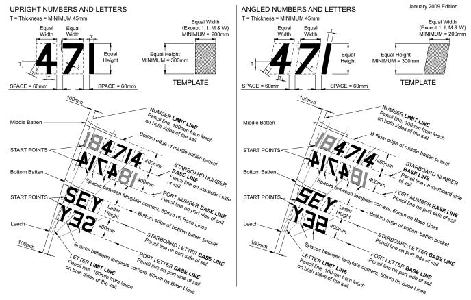
1. MINIMUM SPACE BETWEEN NUMBERS AND LETTERS IN THE CLASS RULES IS 50mm, SO USE 60mm TO ENSURE THAT ANY SMALL ERRORS IN POSITION ARE STILL LEGAL. 2. LAST FOUR DIGITS OF SAIL NUMBER TO BE ONE DARK, DISTINCTIVE COLOUR OR BLACK. PRECEDING DIGITS TO BE A DIFFERENT, CONTRASTING, DISTINCTIVE, COLOUR, PREFERABLY RED. ALL NATIONAL LETTERS TO BE ONE COLOUR. THEY MAY BE ONE OF THE COLOURS OF THE SAIL NUMBER DIGITS OR ANOTHER DISTINCTIVE COLOUR. © ILCA
