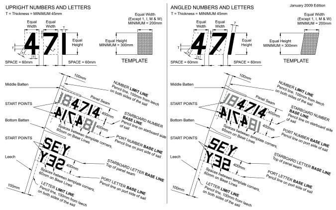
1. MINIMUM SPACE BETWEEN NUMBERS AND LETTERS IN THE CLASS RULES IS 50mm, SO USE 60mm TO ENSURE THAT ANY SMALL ERRORS IN POSITION ARE STILL LEGAL. 2. LAST FOUR DIGITS OF SAIL NUMBER TO BE ONE DARK, DISTINCTIVE COLOUR OR BLACK. PRECEDING DIGITS TO BE A DIFFERENT, CONTRASTING, DISTINCTIVE, COLOUR, PREFERABLY RED. ALL NATIONAL LETTERS TO BE ONE COLOUR. THEY MAY BE ONE OF THE COLOURS OF THE SAIL NUMBER DIGITS OR ANOTHER DISTINCTIVE COLOUR,
