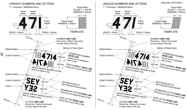
1. MINIMUM SPACE BETWEEN NUMBERS AND LETTERS IN THE CLASS RULES IS 50mm, SO USE 60mm TO ENSURE THAT ANY SMALL ERRORS IN POSITION ARE STILL LEGAL. 2. LAST FOUR DIGITS OF SAIL NUMBER TO BE ONE DARK, DISTINCTIVE COLOUR OR BLACK. PRECEDING DIGITS TO BE A DIFFERENT, CONTRASTING, DISTINCTIVE, COLOUR, PREFERABLY RED. ALL NATIONAL LETTERS TO BE ONE COLOUR. THEY MAY BE ONE OF THE COLOURS OF THE SAIL NUMBER DIGITS OR ANOTHER DISTINCTIVE COLOUR.
