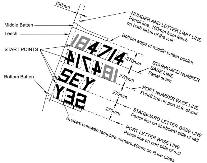
1. MINIMUM SPACE BETWEEN NUMBERS AND LETTERS IN THE CLASS RULES IS 30mm, SO USE 40mm TO ENSURE THAT ANY SMALL ERRORS IN POSITION ARE STILL LEGAL.
