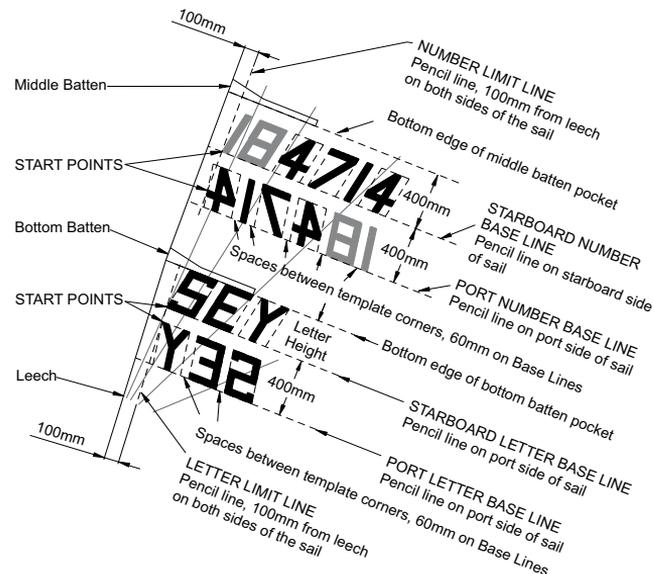
1. MINIMUM SPACE BETWEEN NUMBERS AND LETTERS IN THE CLASS RULES IS 50mm, SO USE 60mm TO ENSURE THAT ANY SMALL ERRORS IN POSITION ARE STILL LEGAL.
