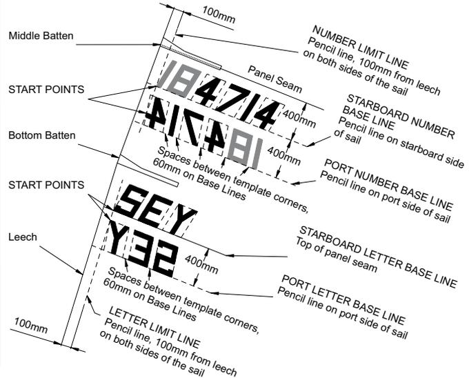
1. MINIMUM SPACE BETWEEN NUMBERS AND LETTERS IN THE CLASS RULES IS 50mm, SO USE 60mm TO ENSURE THAT ANY SMALL ERRORS IN POSITION ARE STILL LEGAL.
